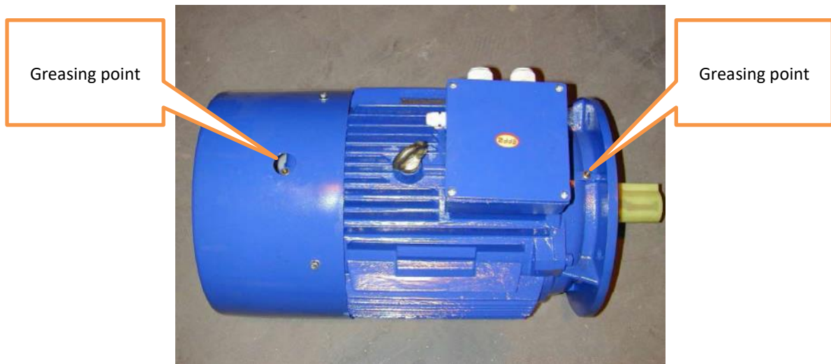
Figure 7-1 – Greasing point electric motors
