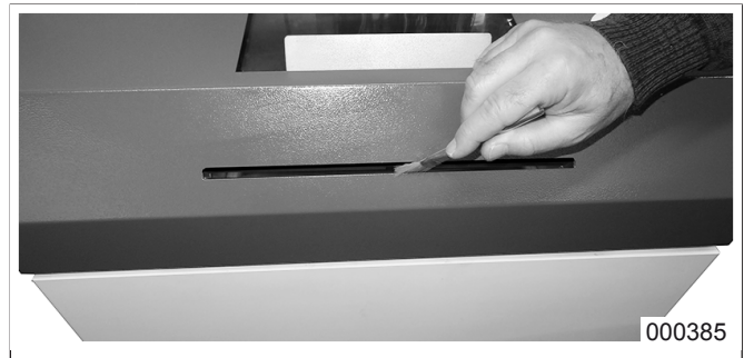
Fig.11 Cleaning the photocells
