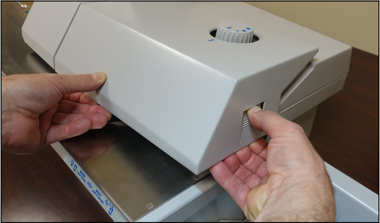
Figure 2-9: Top cover removal interlock triggering
