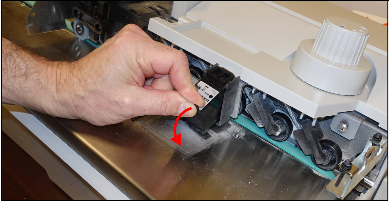
Figure 4-17: Removing the print cartridge
