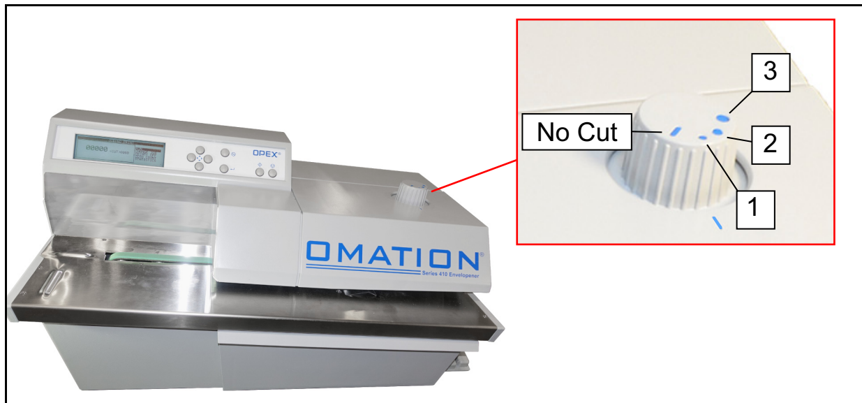
Figure 4-10: Setting the cut depth
