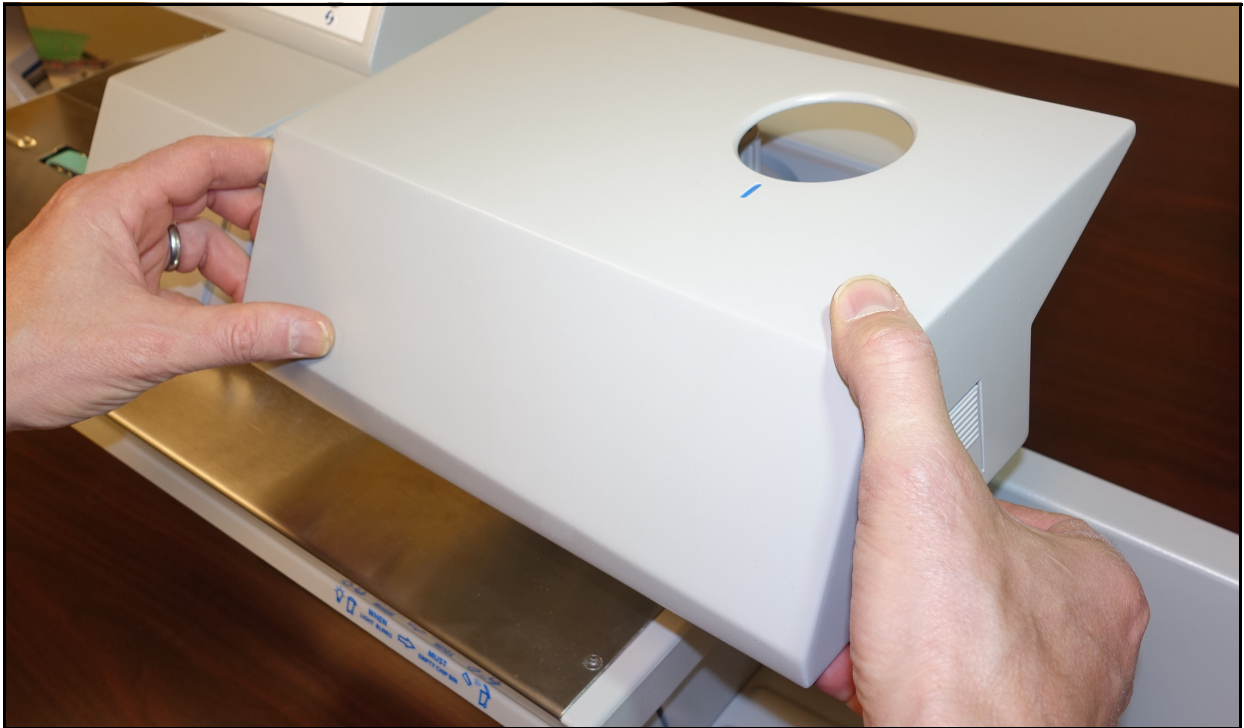
Figure 4-14: Lifting the Nip arm cover
