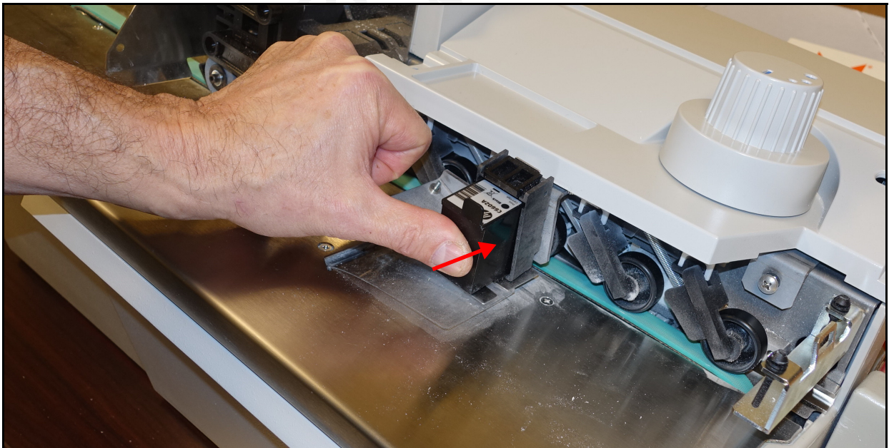
Figure 4-18: Replacing the printer cartridge
