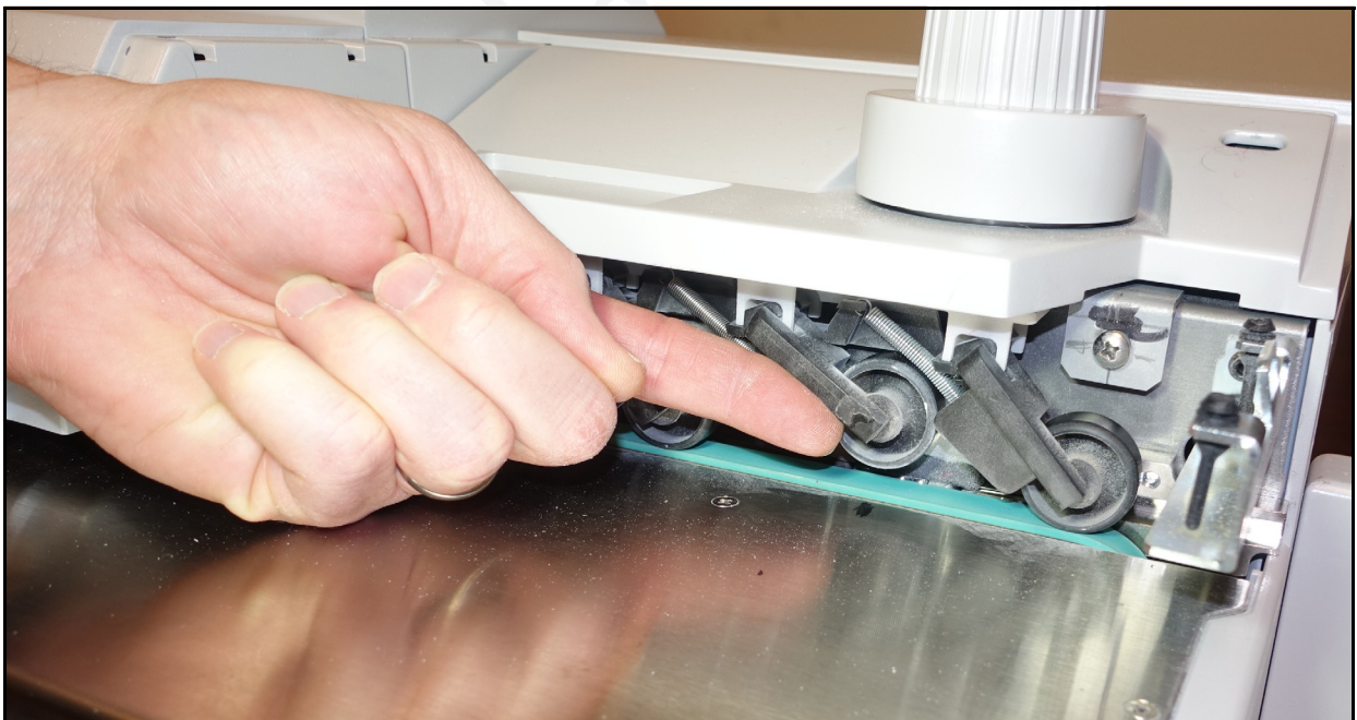
Figure 4-15: Lifting the nip wheels
