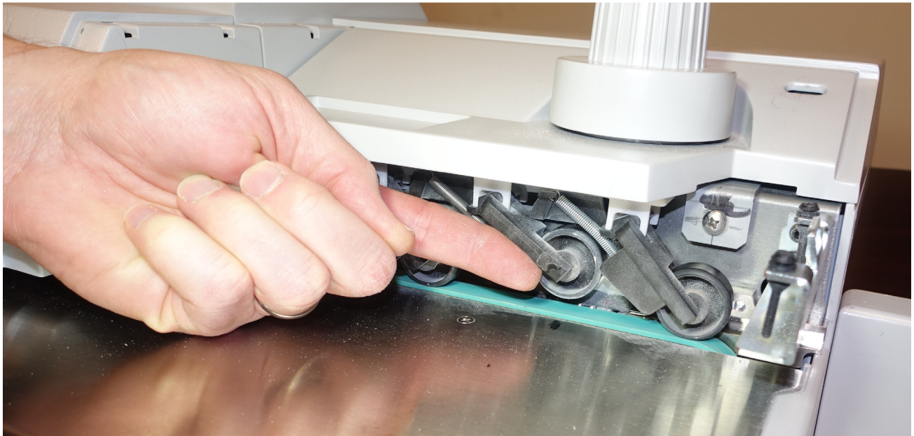
Figure 4-16: Cleaning the nip wheels
