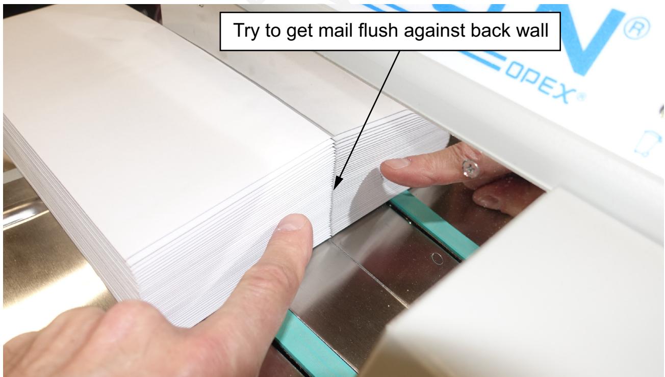
Figure 4-7: Mail flush against Feed Hopper wall
