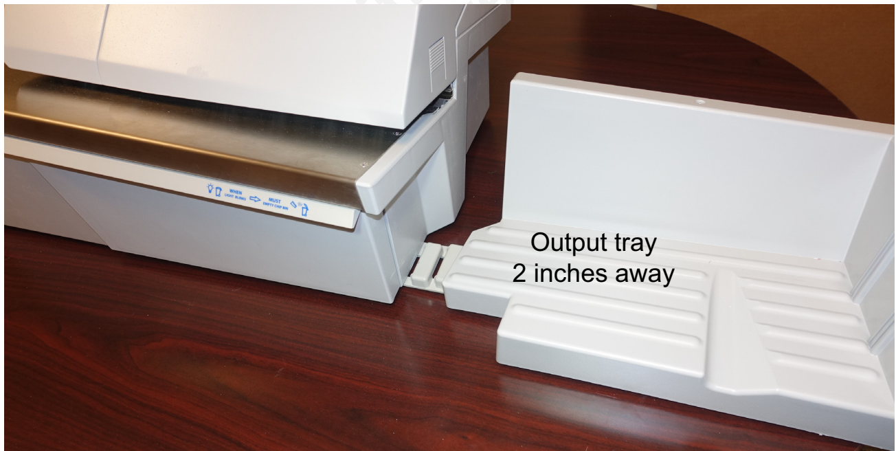
Figure 4-12: Output tray two inches away
