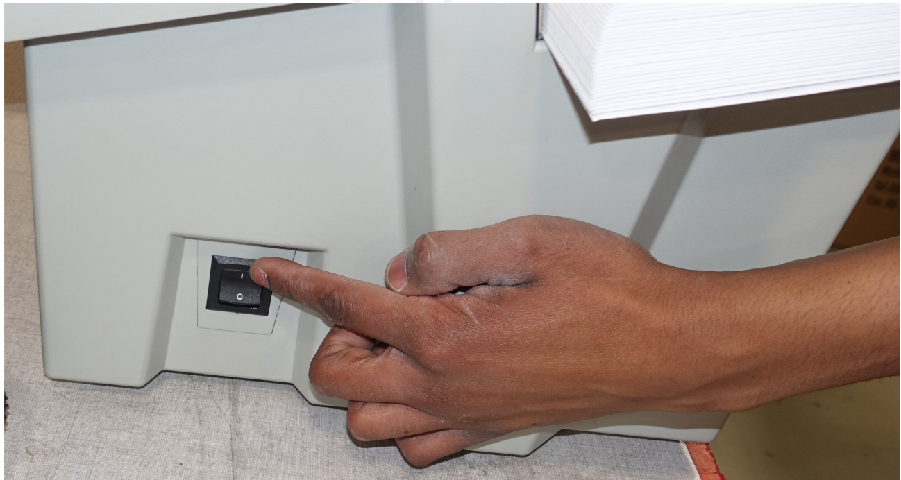
Figure 4-9: AC power switch
