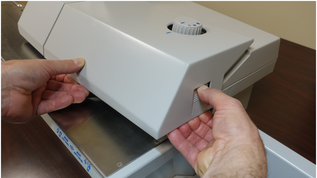
Figure 2-7: Top cover removal interlock triggering
