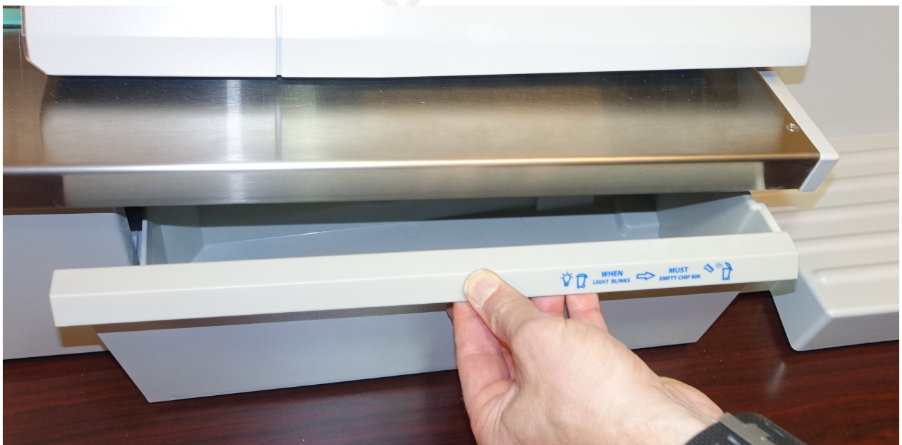
Figure 2-8: Bin tray removal interlock triggering
