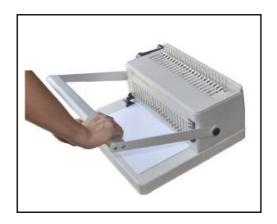
5.Place the plastic rings to the back of comb opening upwards.push the binding handle frontwards to open the plastic rings
