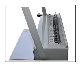
6.Load punched sheets directly onto the open comb
