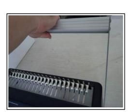
3. Take the punched paper with both hands and insert it directly onto the open rings of the binding element
