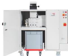
88 liter collecting container with bin-full monitoring
