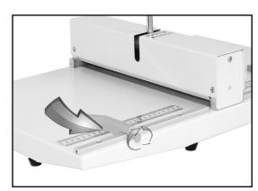
Insert the paper through the perforating device and Ensure the left edge of the paper stay close with the left locator.
