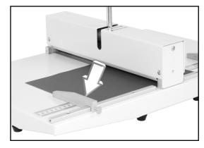
Press the handle to the left till the bottom and release the handle, then put the perforated paper out.
