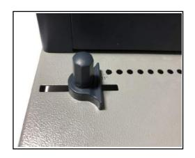
2.Determine the diameter.Put the block under the measuring scale.Push slider downwards.Read the diameter of the binding element.
