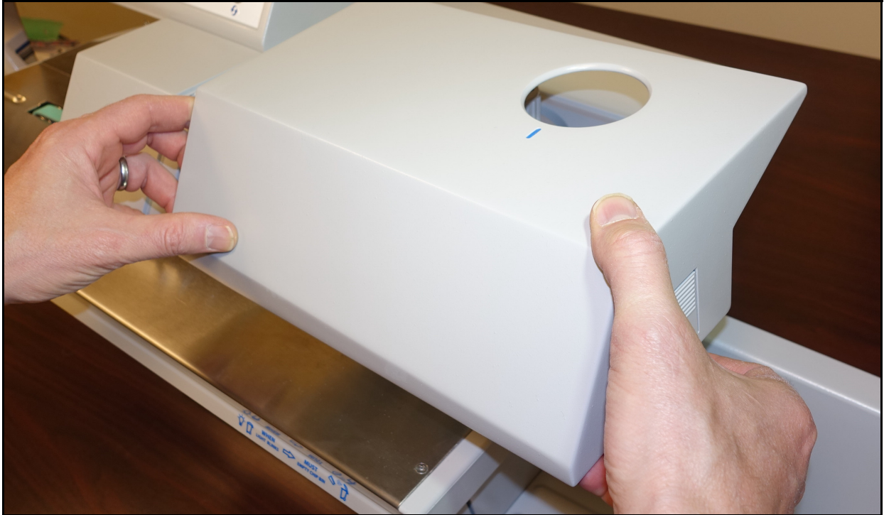
Figure 4-14: Lifting the Nip arm cover
