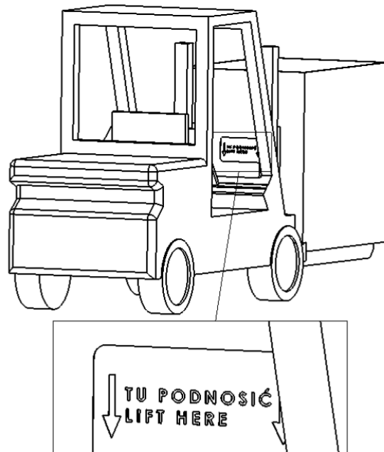
Figure 5a Transporting the cutter in the crate using a forklift.
