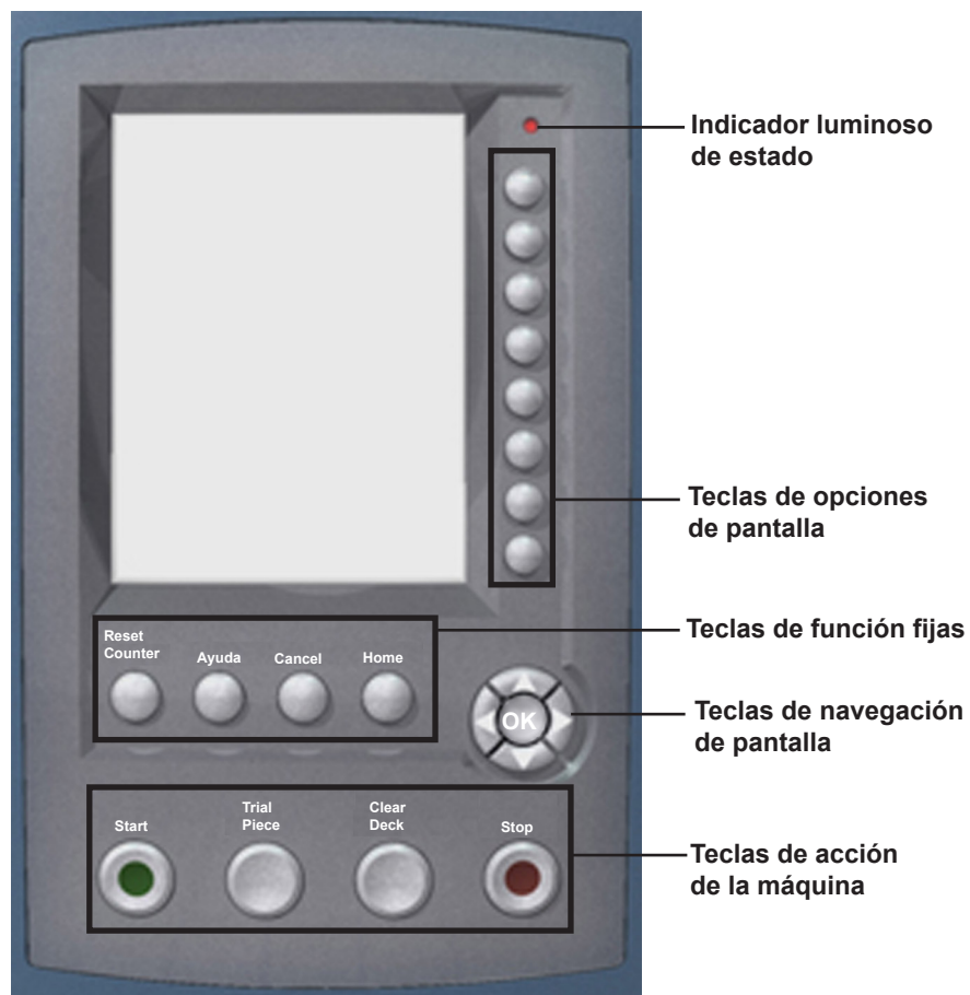
Panel de control
