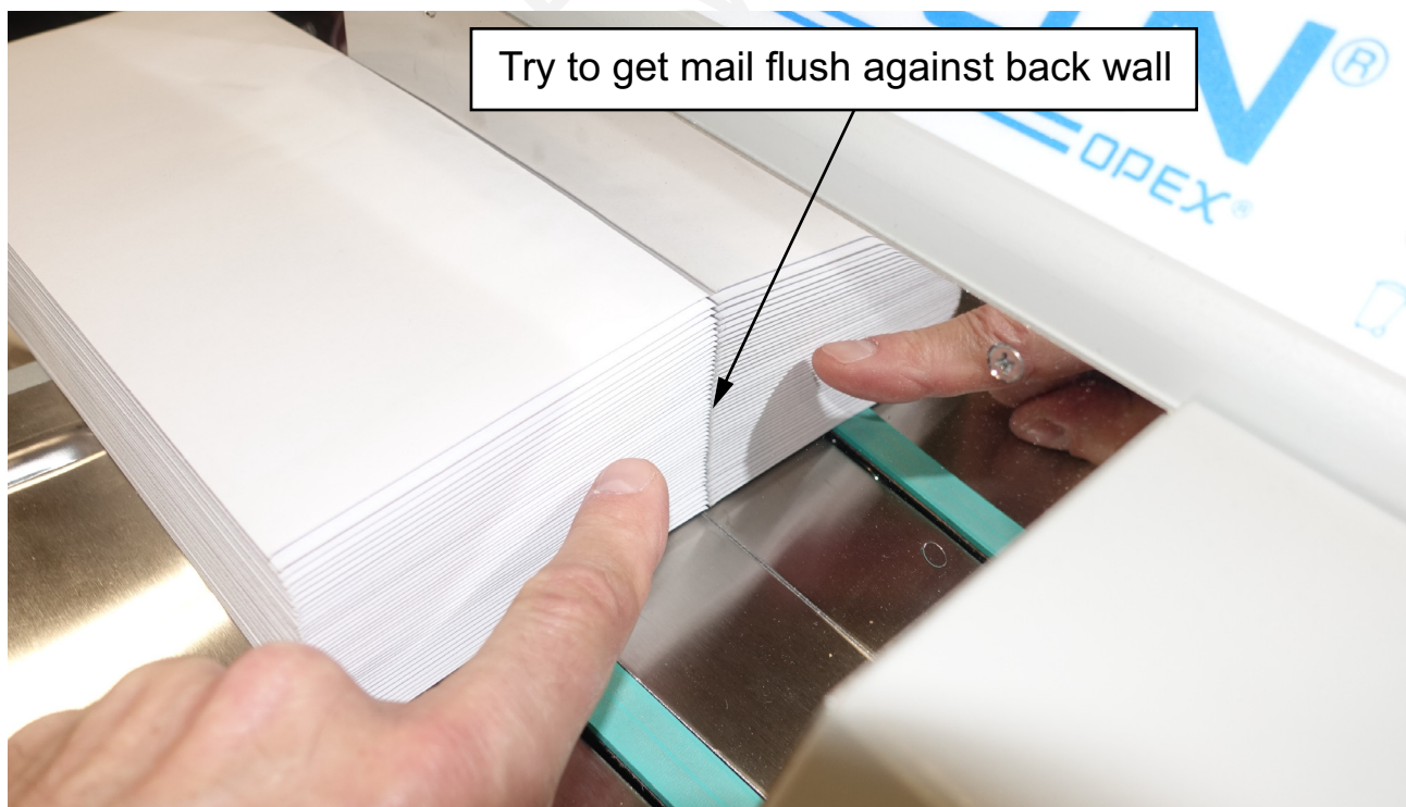
Figure 4-7: Mail flush against Feed Hopper wall
