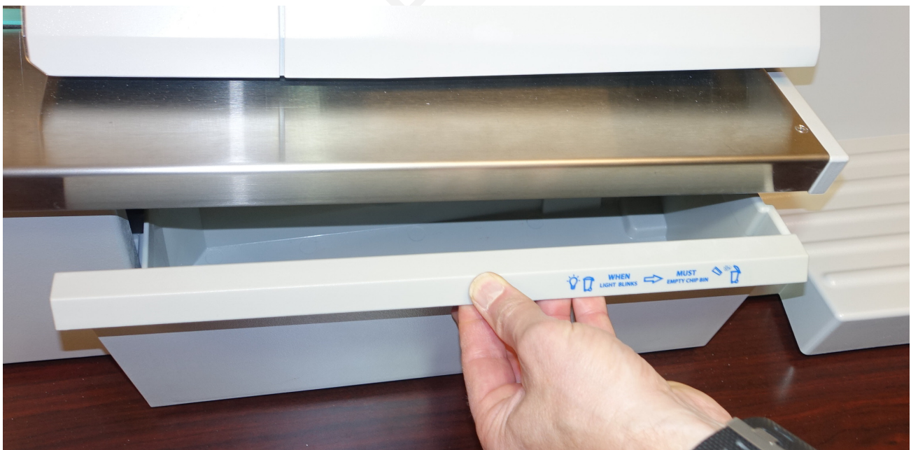
Figure 2-8: Bin tray removal interlock triggering
