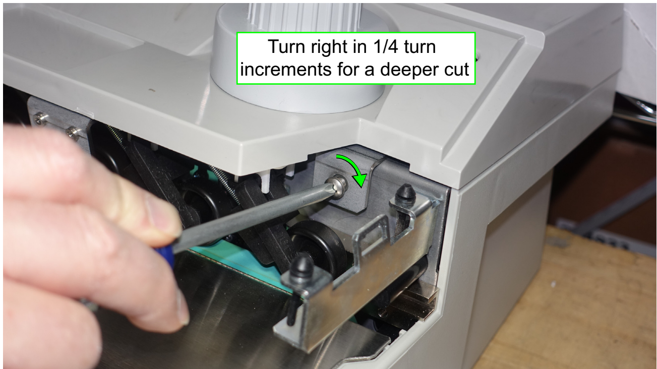
Figure 4-18: Adjusting the cutter depth
