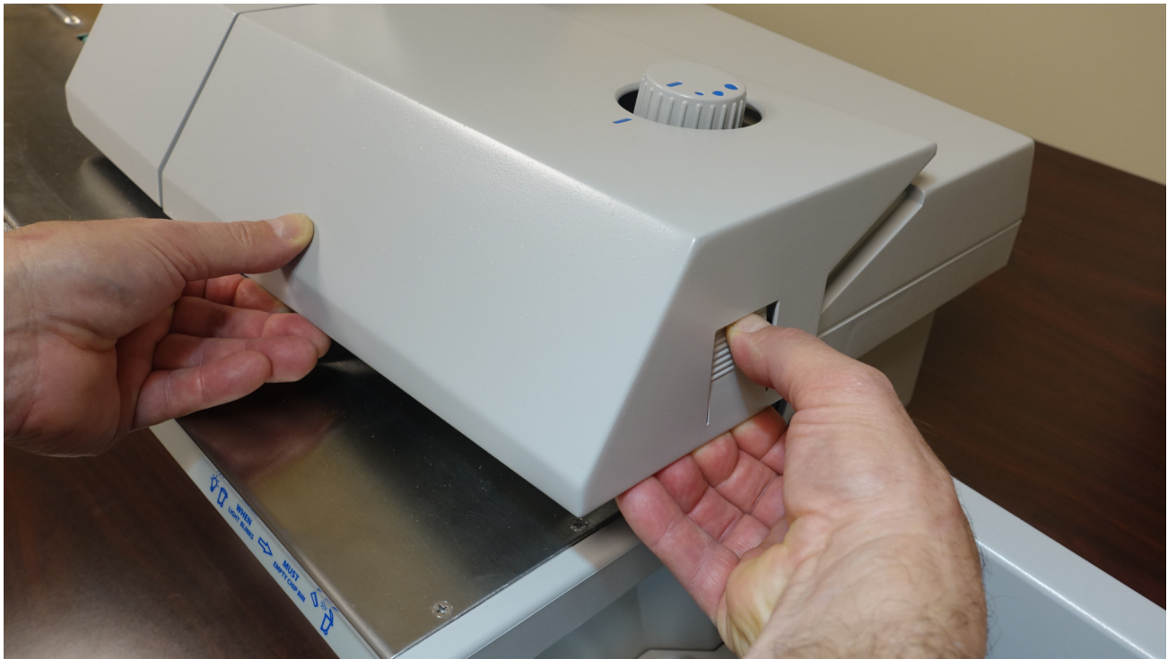
Figure 2-7: Top cover removal interlock triggering
